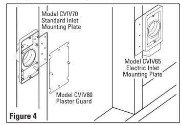
**NOTE:** Installation height will depend on personal preference, but generally the inlet is installed 18" above the finished floor.
